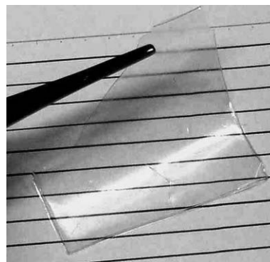
Fig. 8 Photograph of flexible and transparent DNA film. DNA·BF 4 /EtImBF 4 (40 wt%).
